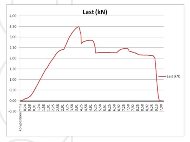
**Comments:** The catch plate was deformed but also the weld was broken in latch.
