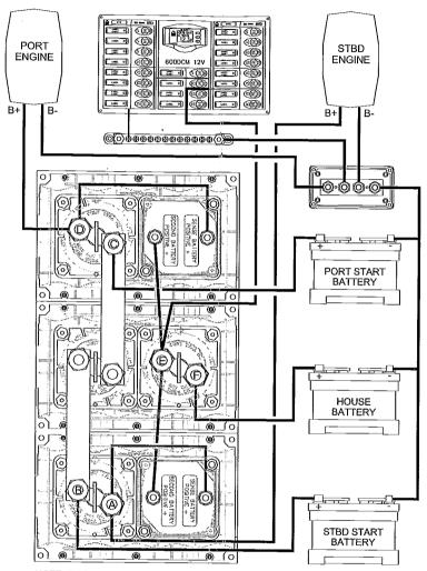
NOTE: THIS DIAGRAM IS NOT INTENDED TO BE A FULL SYSTEMS WIRING DIAGRAM. IT'S SOLE PURPOSE IS TO SHOW CC-803 CONNECTIONS.
