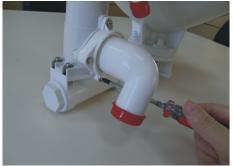
(13) turn the pump unit 180°; put all the screws back and make sure they are tightened.
