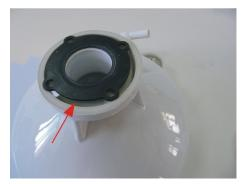
(7) put the rubber gasket back on base unit; make sure to align the screw holes.
