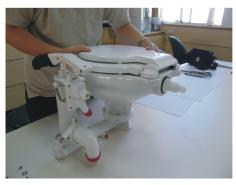
(6) turn the bowl upside down and remove the rubber gasket.
