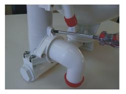
(12) remove the screws x 4 that connecting the pump & base unit.
