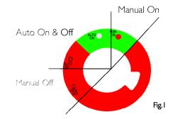
Auto Operation: The 701-MD moves from a state of "Auto Off" to "Auto On" when the remotely mounted switch is turned on. During the time that the battery switch is in "Auto On" mode, the"Auto On" LED is illuminated.
