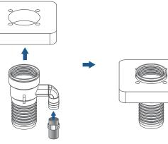
The hose can be attached to the deck fill before installation the fill. Place the body (G) to the cut-out.
