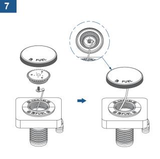
Screw the nylon gear (B) and the cable (C) on the cap (A) by M4 R/H screw (D).
