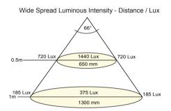
Spread lamps offer higher light intensity while the Wide Spread lens is better for applications with confined spaces or that require extra wide spread of light.
